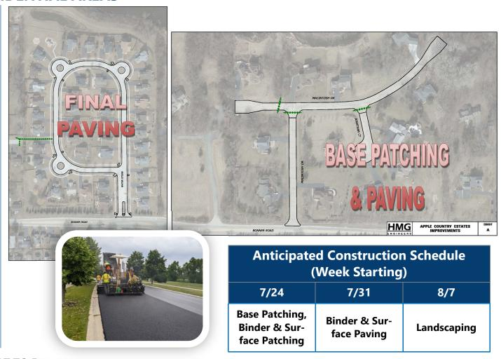
WHAT TO EXPECT: All roads have been milled with base patching scheduled to be completed beginning of this week. Binder asphalt (first layer) will also be installed on all streets by the beginning of this week with surface asphalt (final layer) to follow. An aggregate shoulder is being installed on Wauconda Road to strengthen the pavement edge.
